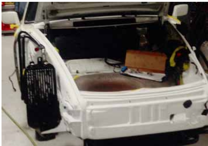
New oil cooler.. almost done
