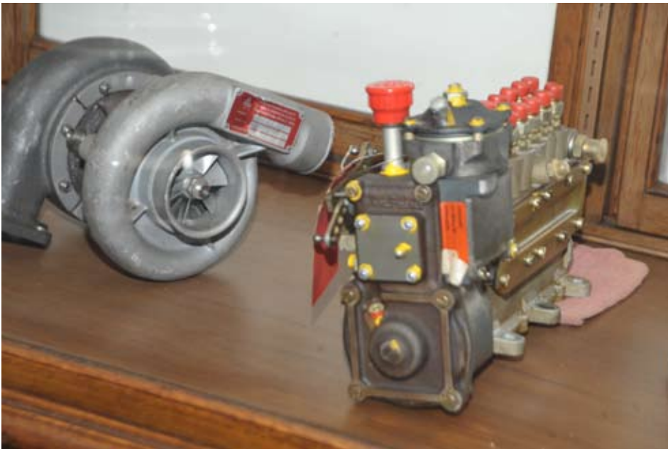
In the jewelry case sits a different kind of jewel. Here the 12 outlet BOSCH injector for 917 sits adjacent to a KKK turbo. Just out of the photo there is a 962 upright.
