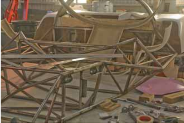
The chassis of 906 #1 taking shape
