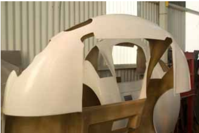
Body panels for the 906 ready for fitting
